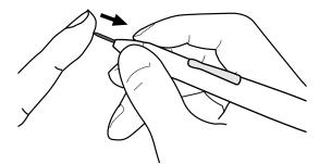
**To insert a new nib:** Slide it straight into the barrel of the pen. Firmly push the nib until it stops. The new nib will slide into the correct position.
